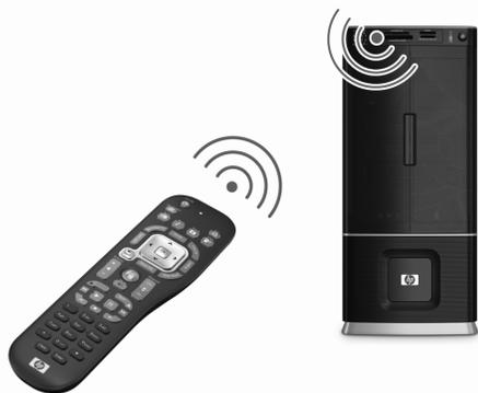
The remote control must be within direct line of sight of the remote sensor, and no farther away than 8 meters (26 feet) apart. The remote control should be no more than 22.5 degrees (45 degrees total) from the center of the remote sensor.
